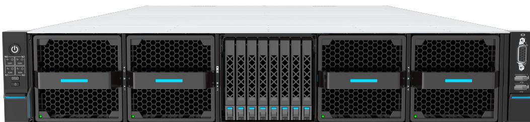
Figure 1-2 K24-X2-A0-R0-00 (8 × 2.5-inch Drive + 4 × 8086 Fan Configuration)
